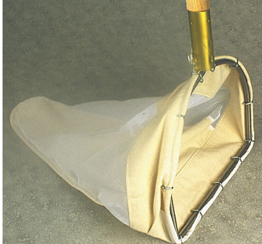
Figure 1. Sampling gear: D-frame kick net.
